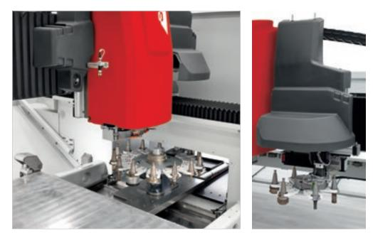
**Tool change up to 10 seconds** The fastest solution in the world of glass, thanks to the 8-position revolver magazine on the head.
