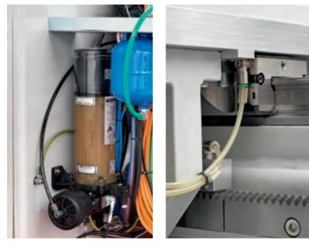
The entire Master range is equipped with an integrated system for the automatic greasing of the movement axes, ensuring constant and precise maintenance every day.
