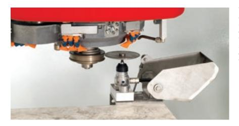
The mechanical pre-setter checks the degree of wear on the diamond tools (with a frequency set by the machine operator) and automatically updates the tool parameters in the machine control system, thereby guaranteeing consistent machining results over time and preventing potential errors.
