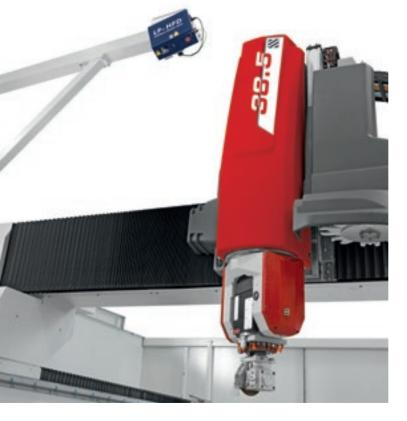
The laser projector is used to made the preparation of the working area quick and easy, reproducing the position of all the suction cups and pieces to be machined on the table and preventing head movements. The on-board laser device allows the panel to be placed on the work table without having to use mechanical stops, ensuring maximum precision with significant time savings. Particularly useful in the presence of large sheets that are heavy and occupy the entire work table.
